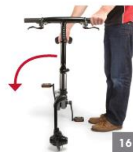
Rotate the pedals to the position demonstrated (right pedal up) and carefully lay the Gocycle flat
