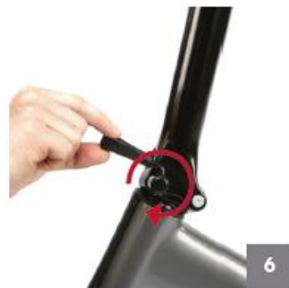
6 Insert the quick release through the handlebar stem and rotate clockwise to tighten
