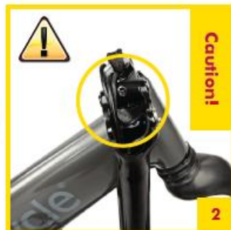
2 Beware of trapping fingers in handlebar folding mechanism!
