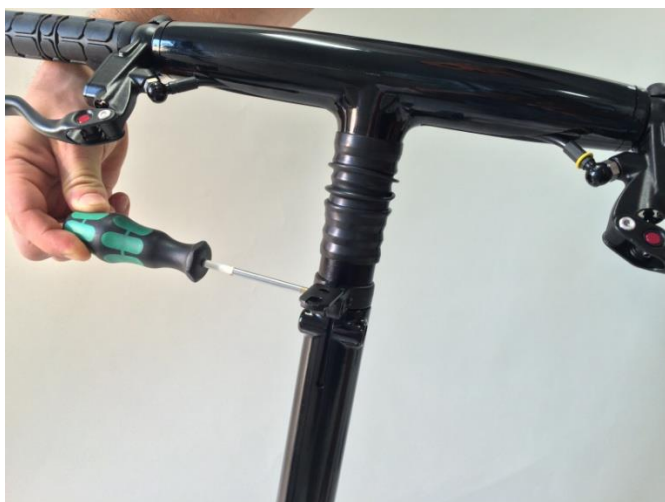
Place the bracket around the upper stem and tighten, using a screwdriver, to secure in the position as shown
