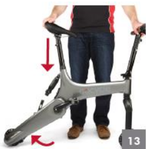
Carefully lower the Gocycle downwards so the Cleandrive continues to rotate backwards
