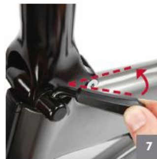
7 The quick release should begin to feel harder to close as it reaches a 90-degree position
