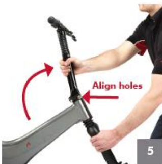
5 Continue to unfold handlebar as shown and align the front hole in the folding mechanism
