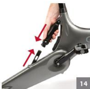
Align the Lockshock™ body with the Lockshock plunger as shown
