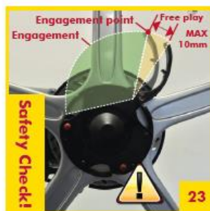
Open and close EACH cam lever to check that it is adjusted and operating as shown. Consult the Owner's Manual if adjustment is needed. NEVER ride with any cam "loose" or if the resistance when closing or opening is not even for all cams.
