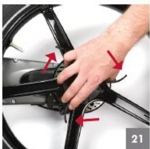
While holding all three cam levers fully open, mount wheel to rear hub
