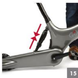
Continue lowering the Gocycle until the Lockshock is fully inserted
