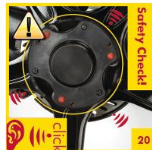
Ensure all cam levers are closed, listening for a "click" from each
