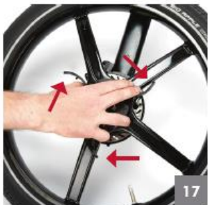
While holding all three cam levers fully open, mount wheel to front hub
