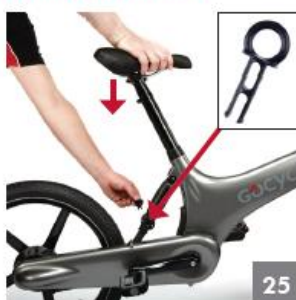
With the Gocycle upright, press down on the saddle and insert Lockshock pin as shown
