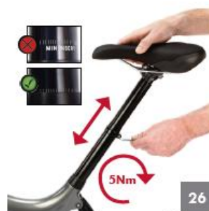
Select preferred saddle height. Tighten the clamp to 5Nm. (DO NOT exceed the minimum insertion mark on the seat post)
