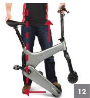
12 Swing the Cleandrive downwards as shown (hint: gently hold your foot on the Cleandrive as you lift the frame as shown)
