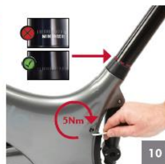
10 Ensuring that the seat post is inserted up to the minimum insertion mark, tighten the securing bolt to 5Nm using a 4mm Allen key
