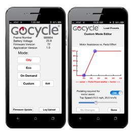
Additional features of the App include the ability to set the legal speed for the rider's local region, remotely view the charge status and health of the Gocycle battery, download the latest software to the Gocycle's controller, and upload the Gocycle's "maintenance log" to KKL's tech support team for remote diagnostics.
