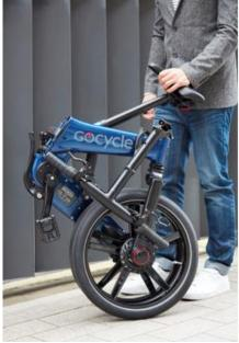
that allows users to monitor battery charge level while on the move. The battery is fully-integrated in the GX's frame for ease of travel and can be quickly removed for charging or maintenance if required.
